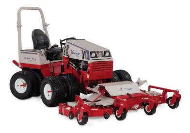
Ventrac's Contour Mower features a 83-inch working width making quick work of any mowing job regardless of the terrain without sacrificing quality of cut. Three independent decks aided by front rollers float along the contour of the ground providing an even cut without scalping, while the rear rollers leave behind a beautiful finish striping pattern. The Contour Mower also features a flip-up deck design.
