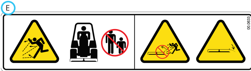
Thrown object hazard. Keep bystanders away from the machine. Do not operate with the deflector belting removed.
