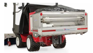
The Ventrac Sidewalk Drop Spreader is the ultimate tool for spreading an array of deicing materials with precision flow control. Designed with a narrow frame and a 40" drop pattern, this spreader is ideal for spreading material on sidewalks and other narrow walkways.
