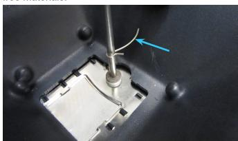
Use a pliers to grab the hook on the rotary agitator and pull the agitator back through the shaft to remove. To reinstall, insert the agitator through the hole in the shaft and push until the hook snaps in place on the shaft. Note the position (sweep) of the agitator and orient correctly when reinstalling.
