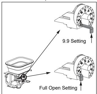
The rate dial has a slot in it at the 9.9 position that will allow the metal guide for the rate gate to slide through. This allows the gate to open fully for spreading mulch and other high volume products.
