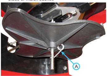
Slide the spinner blade or mulch basket down off the spinner shaft.
