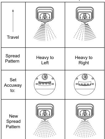
Moving the Accuway plate shifts the material on the spinner. Adjustment is very sensitive and should be done in small increments until the spread pattern is centered.
