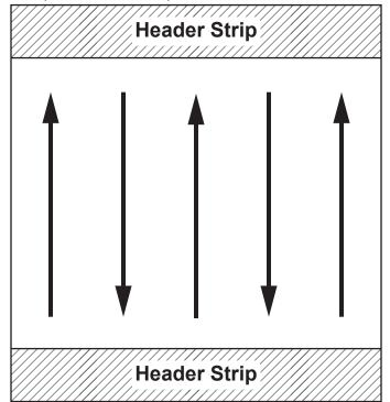
Make the first pass at one-half of the spread width. Make each additional pass at the full spread width.
