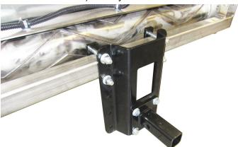
NOTE: Ventrac recommends installing the hitch mount to the spreader using the top set of holes.
