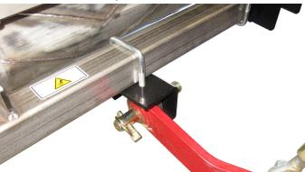
20. Insert the 3 point top link into the channel in the 3 point top link hitch, install the top link pin, and secure with a linchpin.
