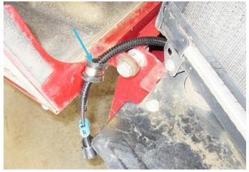
11. Use a zip tie to fasten the wire harness to the battery clamp and tuck any excess wire down into the rear frame.
