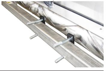
19. Install the spreader hitch mount onto the 4) 1/2 x 3-3/4" bolts and fasten loosely with 4) 1/2" flat washers and 4) 1/2" nylon lock nuts.
