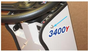
4. Place a 1/4" flat washer onto the 1/4 x 3/4" flange bolt and insert the flange bolt through the hole in the control box mount bracket. Place another 1/4" flat washer onto the flange bolt and install in the right upper hole of the steering column cover with the flange of the control box mount bracket
