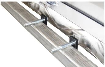
10. Insert a 1/2 x 3-3/4" bolt into the bottom hole on both of the small hitch plates.
