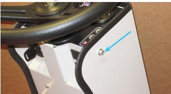
4. Place a 1/4" flat washer onto the 1/4 x 3/4" flange bolt and insert the flange bolt through the hole in the control box mount bracket. Place another 1/4" flat washer onto the flange bolt and install in the right upper hole of the steering column cover with the flange of the control box mount bracket hooked over the top edge or the steering column cover. Torque to 100 in-lbs (11 Nm).
