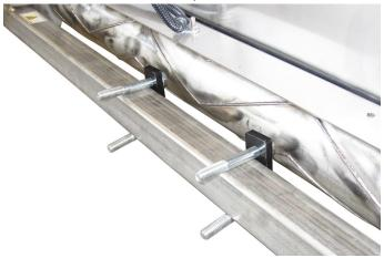
11. Install the spreader hitch mount onto the 4) 1/2 x 3-3/4" bolts and fasten loosely with 4) 1/2" flat washers and 4) 1/2" nylon lock nuts.
