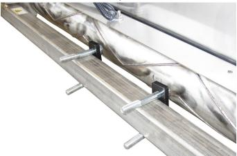
10. Install the spreader hitch mount onto the 4) 1/2 x 3-3/4" bolts and fasten loosely with 4) 1/2" flat washers and 4) 1/2" nylon lock nuts.
