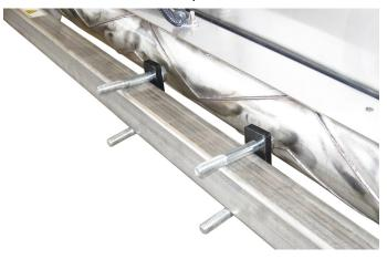
5. Install the spreader hitch mount onto the 4) 1/2 x 3-3/4" bolts and fasten loosely with 4) 1/2" flat washers and 4) 1/2" nylon lock nuts.
