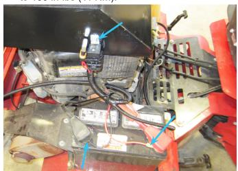
Connect the wire harness to the battery with the red wire attaching to the positive terminal and the black wire attaching to the negative terminal. 5. Remove the white wire with red stripe from position F on the fuse panel.
