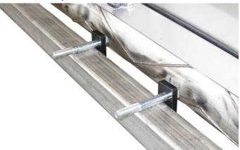
18. Insert a 1/2 x 3-3/4" bolt into the bottom hole on both of the small hitch plates.
