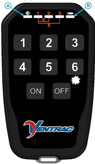
Press and hold the On button until the power on indicator flashes (approximately 1 second) to turn on the control unit.
