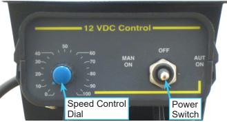
Power is sent to the motor by moving the switch to either MAN ON or AUT ON. Moving the switch to the MAN ON position disregards the speed control dial and sends full power to the motor. Moving the switch to AUT ON allows the motor speed to be controlled by the speed control dial setting.
