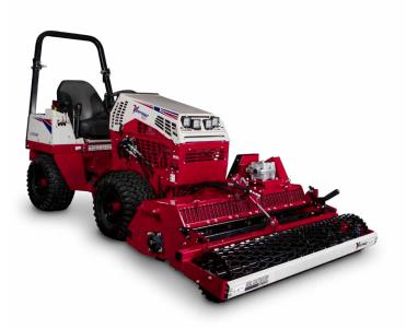
The DC520 Soil Cultivator prepares bare soil by cultivating a soft and uniform seedbed for the best possible direct-seeding results. This attachment works well to recondition hard, compacted soil into a better surface for more successful and consistent germination rates.
